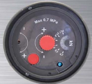
Easy to use pressure setting adjustments and hydraulic oil level indicator make this an intuitive tool to use
